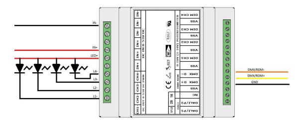
In this mode (configuration pre-set in factory), the device can be controlled through a DMX-512/RDM bus.
