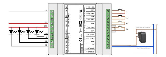
In this mode it is possible to control the 4 output channels by pressing 4 normally open keys (buttons). The buttons must be connected to the VSS and DIM CH1 terminals for channel 1, to VSS and DIM CH2 for channel 2 and so on.
