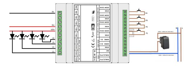
In this mode, the driver works as a generator of pre-programmed DMX shows, with input on 4 N/O buttons connected as shown: on the VSS and DIM CH1 terminals - P1 button, on the VSS and DIM CH2 terminals - P2 button and so on.
