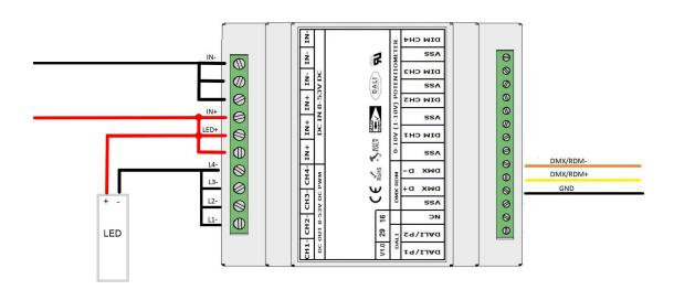
In this mode, the device can be controlled through a DMX-512/RDM bus with single channel working. The channel outputs are bridged with each other.
