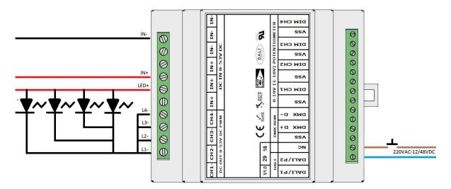
In this mode it is possible to synchronously control the 4 output channels by pressing a NO button connected as shown.
