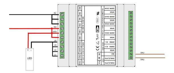
In this mode, the device works as a 4 channels DALI dimmer. The maximal current the DALI bus absorbs is of almost 2mA.
