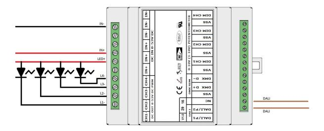
In this mode, the device works as a 4 channels DALI dimmer. The device is recognised during addressing as 4 totally independent DALI devices totally independent. The maximal current the DALI bus absorbs is of almost 2mA.
